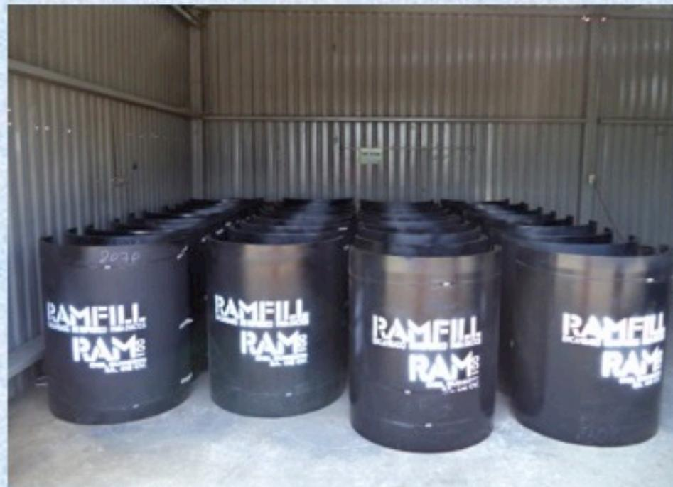
FABRICADAS A PARTIR DE PLACA DE ACERO ASTM O TUBERIA API CERTIFICADOS, CON LA MISMA O MAYOR RESISTENCIA A LA TENSION DEL DUCTO A REPARAR
